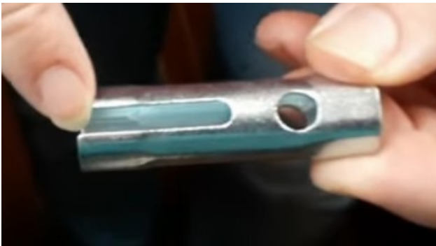
Glow plug extraction tool
